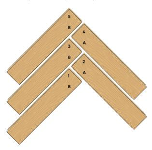
Install the boards precisely and in the order indicated by the numbers on the boards. Carefully check the joints between the planks after every plank which is added. No protruding edge may be felt!
