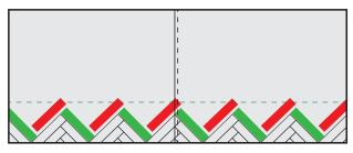
This alternating installation of A-planks and B-planks continues throughout the whole room. It is important to check frequently that:
