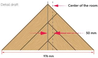
In case you have calculated and built an uneven number of triangles, leave the outer two triangles aside. For the case that you have built an even number of triangles, lay one aside. Lay out the middle triangles with their long side towards the starting wall. Make sure the underlayment is installaed beforehand and the installation line remains visible.
